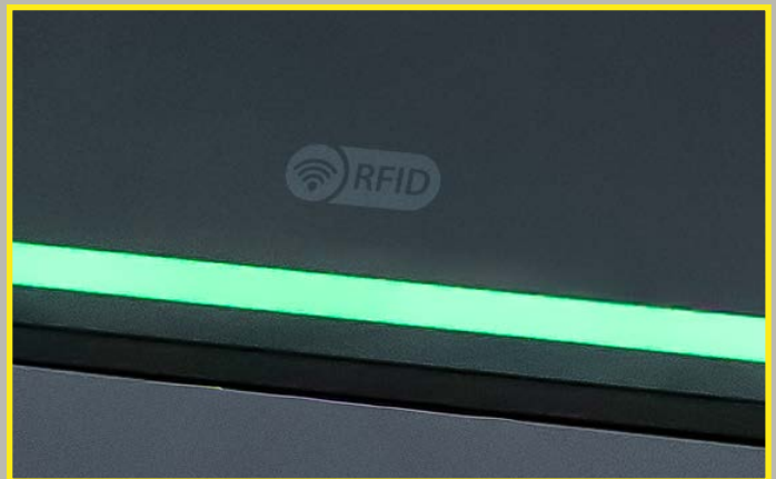
RFID sensor for convenient login and logout with dinoChip
